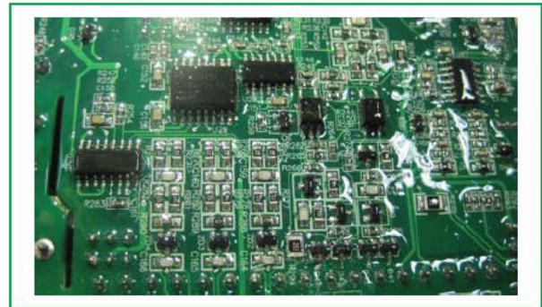
Thick PCBA coating for hard environment using
